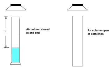
A closed end of a tube must always be a node and an open end of a tube must always be an anti-node
