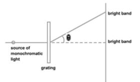
The diagram above illustrates the effect of a grating on a monochromatic source of light. For any particular grating *d* is constant and sin  $\theta$  depends only on wavelength and so the bigger the wavelength the bigger the angle  $\theta$  (hence why red is further from the central maxima).
