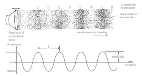
The vibrations of the loudspeaker set up a series of compressions and rarefactions in the air. The graph of air pressure as a function of distance from the speaker is a sine curve.
